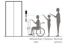
Buttons shall be placed at a height that is convenient for visually impaired person, children and wheelchair user. Recommend button height (H1 ~ H2): 900mm ~ 1100mm.
