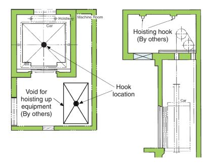
When building contractor provides the temporary void on the machine room floor for hoisting up elevator equipment, building contractor shall provide an additional suspension hook, positioned directly above the center of the void. (For details, please consult with Hitachi.)
